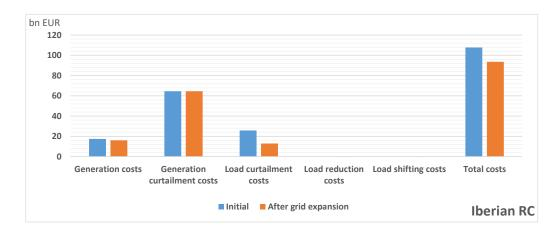
It can be seen, that even though there is a small increase in generation curtailment costs, the significant reduction of the total costs is due to the reduction of the load curtailment costs (almost 50% reduction) and generation costs (8%).
