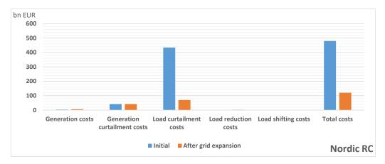
Such a significant reduction in initial costs was made possible by a very significant reduction in the load curtailment costs (reduction of almost 84%).
