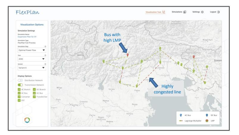
**Step 2**: visualize the results of the non-expanded optimal power flow with, in particular, congested lines and buses with high locational marginal prices
